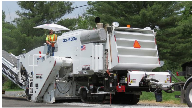
Figure 2. CIR Milling Process (Roadtec, 2019)
