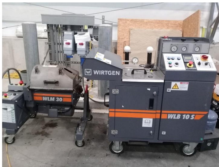
Figure 11. Laboratory-Scale Foaming Machine
