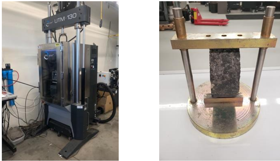
Figure 17. Indirect Tensile Strength Test
